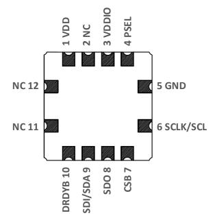
Fig. 3 Pin configuration (Bottom view)
