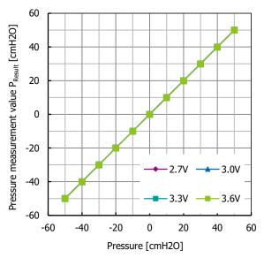
Fig. 23.2 Pressure measurement value P<sub>Result</sub> supply voltage characteristic
