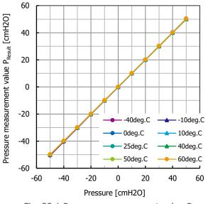
Fig. 23.1 Pressure measurement value P<sub>Result</sub> temperature characteristic
