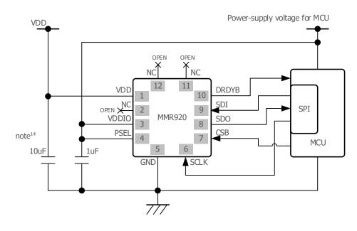
Fig. 20 Typical Electrical Connection (SPI)
