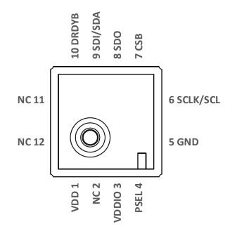
Fig. 2 Pin configuration (Top view)
