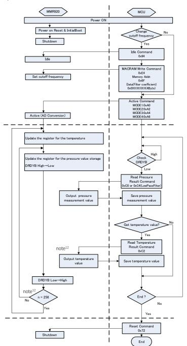
Fig. 7 Flow chart of pressure/temperature measurement
