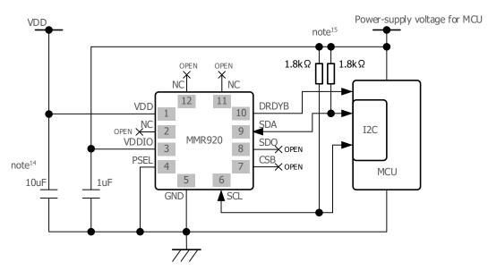
Fig. 21 Typical Electrical Connection (I2C)
