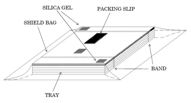
THESE 6 TRAYS WHICH ARE 5 TRAYS WITH PRODUCTS AND EMPTY TRAY AS LID ARE PILED UP. ALSO, THESE TRAYS ARE FIXED BY BAND. THESE ARE VACUUM-HEAT-SEALED TOGETHER WITH THE SILICA GEL. %THIS TRAY HAS TYPE A AND TYPE B. THEY ARE PILED UP ALTERNATELY. (IT IS POSSIBLE TO USE BOTH TYPE TRAYS AS EMPTY ONE.)
