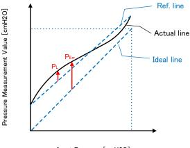
Input Pressure [cmH20] Fig. 4 Definition of Characteristics
