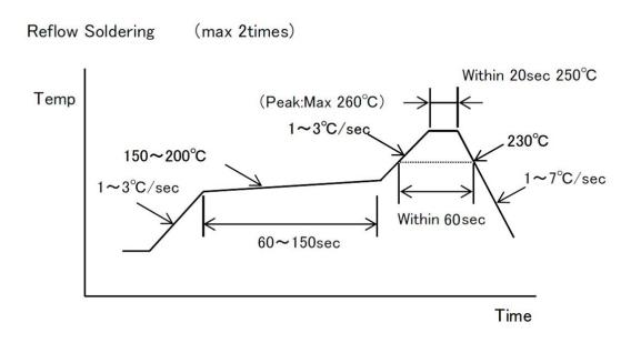
This profile gives recommended values, which are not guaranteed. For mounting the package, evaluate the profile with the equipment, conditions, and materialsto be used.
