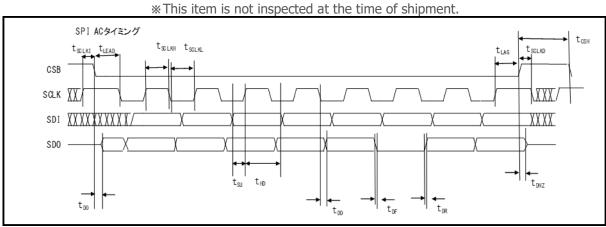
Fig. 11 SPI AC timing chart
